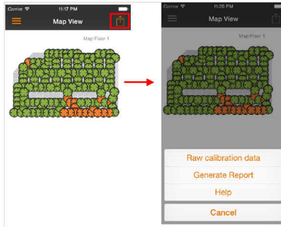
Figure 77: Click the Options icon to access the Help, Generate Report and Raw Calibration Data tools
